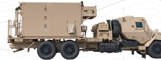
1.1 – Engagement Operations Center (EOC) S-280 Shelter
